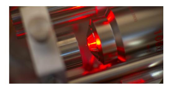
A microscope objective (right) focuses laser light to create the optical tweezers in which a nanosphere (tiny red dot in the centre of the image) is levitated. Credit: ETH Zurich / Erik Hebestreit and Vijay Jain
