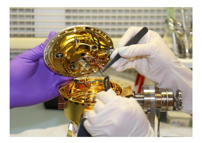
LLNL scientists perform assembly work on a prototype gamma-ray spectrometer that is undergoing tests as part of an effort to design and build an instrument to fly aboard a NASA mission to the 16 Psyche asteroid. Credit: Carrie Martin
