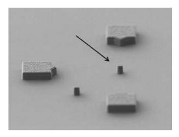
Oblique angle scanning electron microscopy image of a 500 nanometer diameter microdisk. Credit: A\*STAR Data Storage Institute
