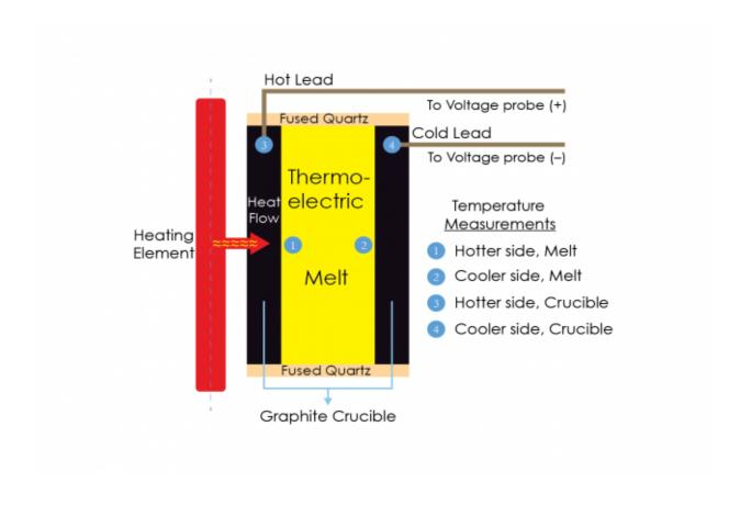
MIT researchers have demonstrated a liquid thermoelectric device with a molten compound of tin and sulfur that can efficiently convert waste heat to electricity, opening the way to affordably transforming waste heat to energy conversion at high temperatures. Blue circles are sites of temperature measurements in the molten liquid, hot side (1), cooler side (2), and in walls of the crucible (heat-resistant pot) hot side (3) and cooler side (4). Credit: Youyang Zhao
