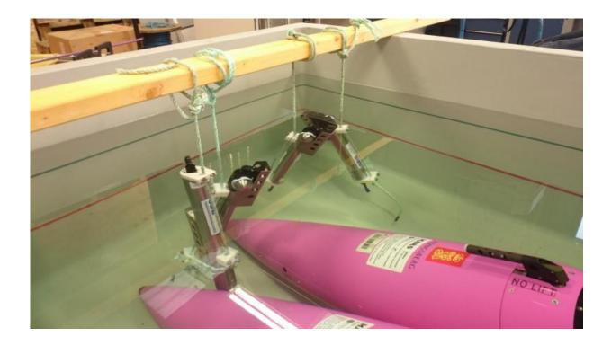
Testing new oxygen sensors (combined with sensors to measure temperature, salinity and pressure) at SAMS' Scottish Marine Robotics Facility, alongside two of its gliders. Credit: Estelle D
