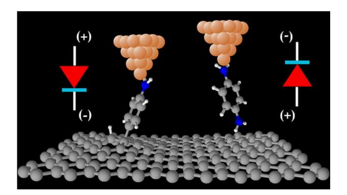
The researchers performed the characterization of graphene-based molecular electronic devices at room-temperature and demonstrated that molecules covalently attached to mechanically robust graphene substrates are ideal candidates for next-generation molecular electronic devices. Credit: Alexander Rudnev, University of Bern
