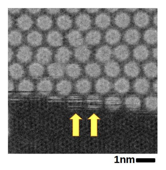
Scanning transmission electron microscope image of a fullerene layer between two graphene sheets. Due to the motion of the fullerenes at the edge, they are only partially visible. Credit: Kimmo Mustonen/ Jannik Meyer, Universität Wien
