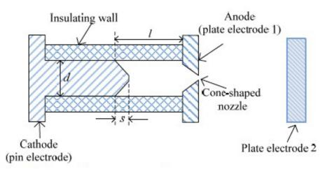
A diagram of the mechanical structure of the capillary. Credit: Li/Xiong/Cheng/Peng/Pan
