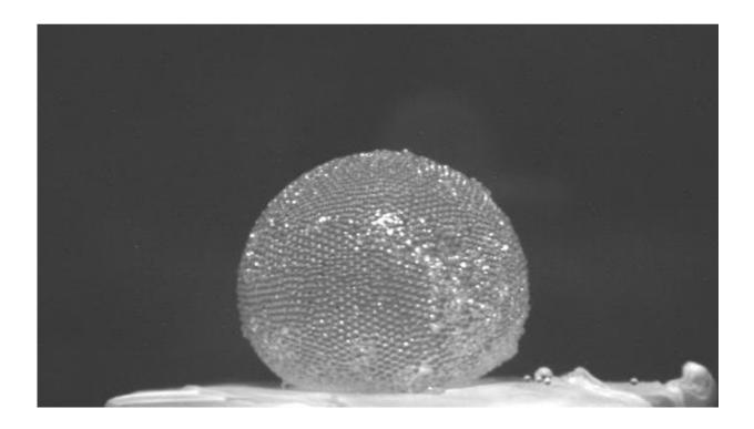
Hard outside, soft inside. The plastic shell of a gas marble can withstand at least 10 times atmospheric pressure, with no volume increase. Credit: Y. Timounay/UPE, via *Physics*
