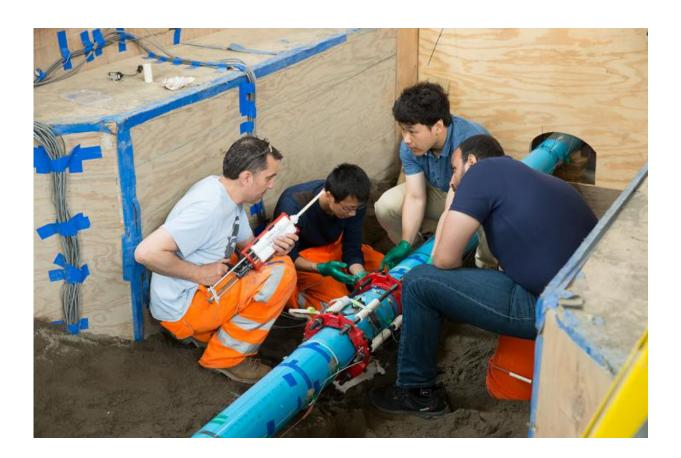
Researchers from the Cambridge Centre for Smart Infrastructure and Construction glue fiber-optic sensors to a test pipe in Cornell's Geotechnical Lifelines Large-Scale Testing Facility. Credit: Cornell University
