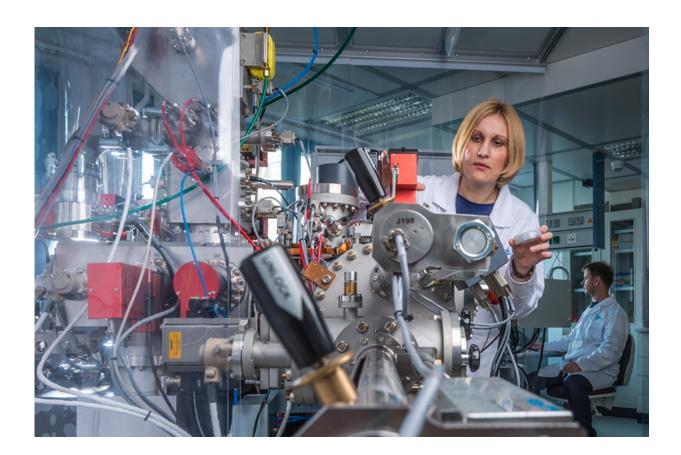
The NanoSIMS is a secondary ion mass spectrometry system with a spatial resolution of down to 50 nanometres. This high resolution combined with its mass sensitivity make it possible to detect elements and isotopes on cell surfaces and chemical changes inside cells. This instrument is part of the newly established research platform, ProVIS. Dr. Niculina Musat and Dr. Hryhoriy Stryhanyuk (co-authors of the paper) during sample analysis. Credit: UFZ
