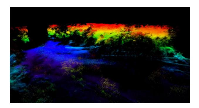
Specially designed laser system and a new methodology based on gated digital holography enable LiDAR to see through obscuring elements like foliage and netting. Credit: US Naval Research Laboratory
