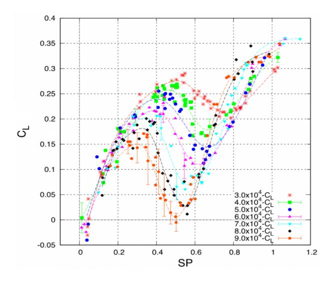
Lift coefficient as a function of the spin parameter SP. Credit: University of Electro-Communications
