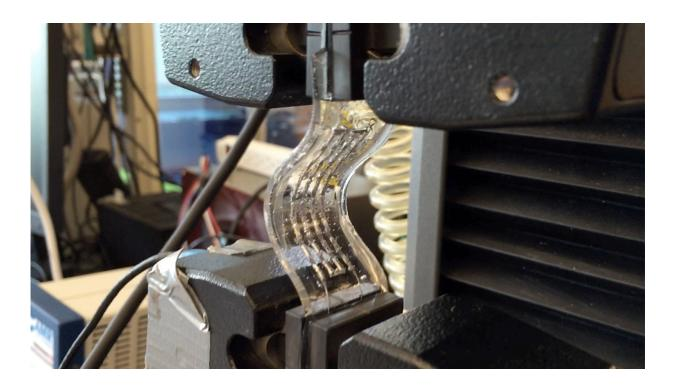
NC State's thermoelectric harvester has the material quality of rigid devices inside a flexible package. Credit: Mehmet Ozturk, NC State University.
