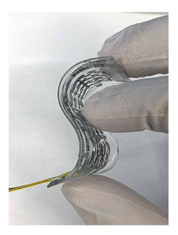
Liquid metal in the flexible thermoelectric device allows for self-healing. Rigid devices do not have the ability to heal themselves. Credit: Mehmet Ozturk, NC State University.
