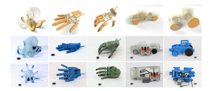
Carious results of the algorithm. The middle and bottom row show objects that have been fabricated by the researchers using 3-D printing. Credit: IST Austria
