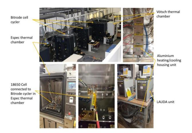
The long-term battery ageing test set up at WMG's Energy Innovation Centre. Credit: University of Warwick
