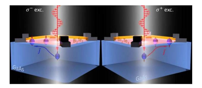
The researchers have taken the first step towards transferring spin-oriented electrons between a topological insulator (orange layer) and a conventional semiconductor (blue layer). Credit: Linköping Universitet
