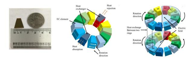
(Left) Photograph of one of the twelve electrocaloric elements that form a ring. (Right) Illustration of the electrocaloric device with rotating rings. Credit: Zhang et al. ©2017 American Institute of Physics
