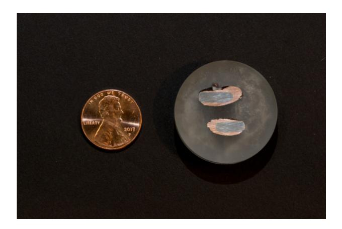
A new penny, at left, contrasts with samples of nearly pure copper deposited on an iron electrode after extraction through an electrochemical process. Credit: Denis Paiste/Materials Processing Center
