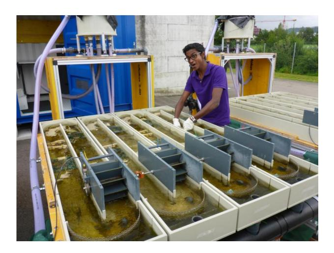
A 16-channel flume system was used to study the effects of different constituents of wastewater. Credit: Eawag
