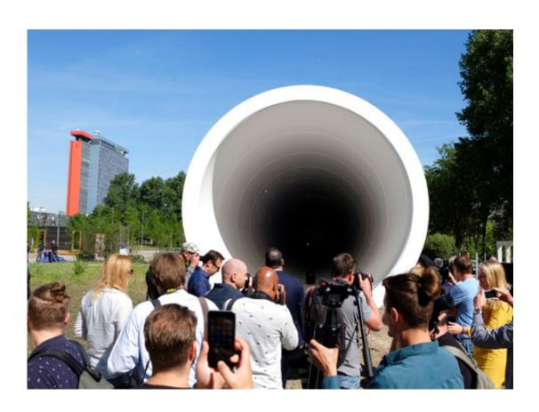
People look at a hyperloop test facility unveiled by a tech startup and a construction company in Delft, Netherlands, Thursday, June 1, 2017. The 30 meter (100 foot) long white steel tube will be used to help develop the futuristic high-speed transportation system. The tube is a first step toward developing the system in the Netherlands, a key European transportation transport hub. (AP Photo/Mike Corder)
