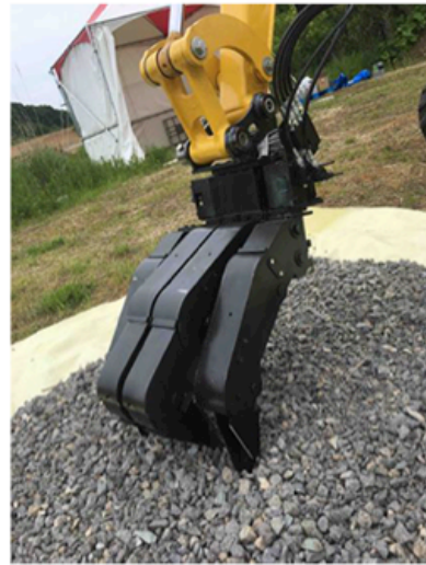
Gravel digging with shovel mode
