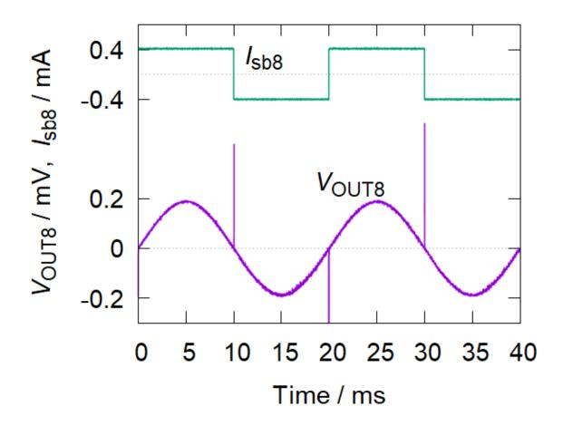
Sinusoidal waves indicative of bipolar outgoing voltages generated using the 8-bit variable pulse number multiplier. Credit: University of Electro Communications
