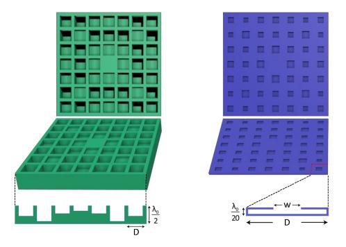
A conventional, two-dimensional conventional Schroeder diffuser (on the left), compared to a new, 'ultra-thin' two-dimensional Schroeder diffuser (at right). The ultra-thin diffuser is 10 times thinner. Credit: Yun Jing
