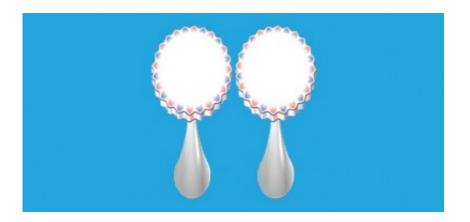
Numerical simulation of acoustic waves propagating at the edges of microdisks. Deformations represent movements caused by acoustic waves. The false color scale represents the intensity of the light electromagnetic field on the disk surfaces. Credit: Gustavo Silva Wiederhecker
