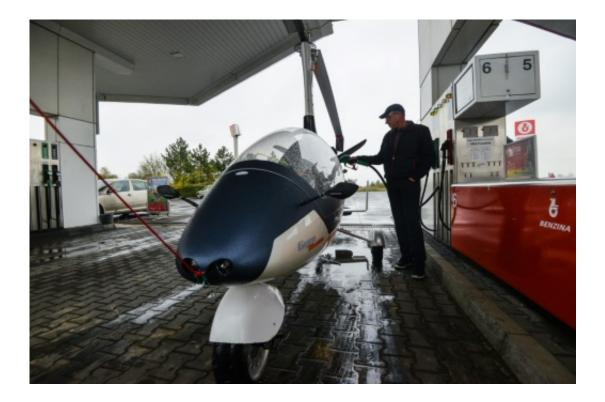
Pavel Brezina's GyroDrive vehicle is based on a gyroplane—a minihelicopter—that uses a copter-style rotor to move up and down, and an aeroplanetype "pusher propeller" to go forward.
