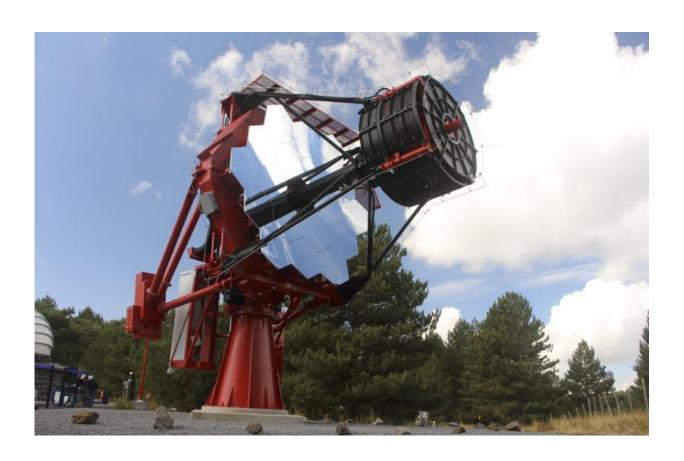
The ASTRI is one of three Small-Sized Telescope (SST) designs being prototyped. SSTs will outnumber all the other telescopes with 70 planned to be spread out over several square kilometers in the southern hemisphere array only. This is because very high-energy gamma-ray showers produce a large amount of Cherenkov light, and the SST is sensitive to the highest energy gamma rays (between a few TeV and 300 TeV). Credit: CTA Collaboration
