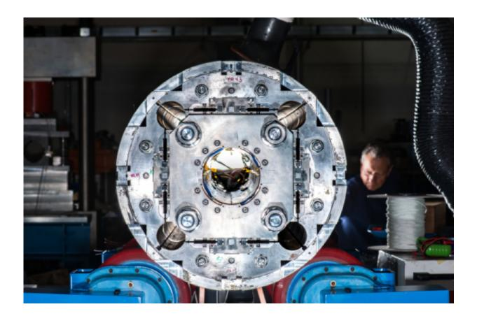
View of the cross-section of a short-model magnet for the High Luminosity LHC quadrupole, with three coils manufactured at CERN and one coil made in the US. Credit: Robert Hradil, Monika Majer/ProStudio22.ch
