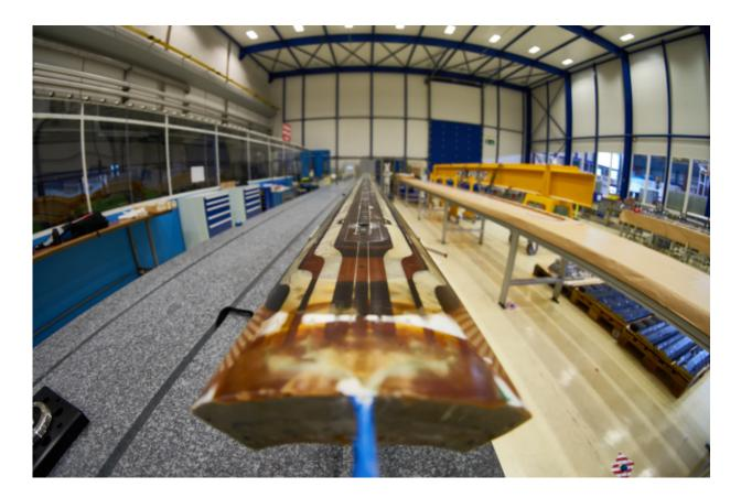
The new 7.15-metre-long coils for the Nb3Sn quadrupoles for HL-LHC, in the Large Magnet Facility building. Credit: M. Brice/CERN
