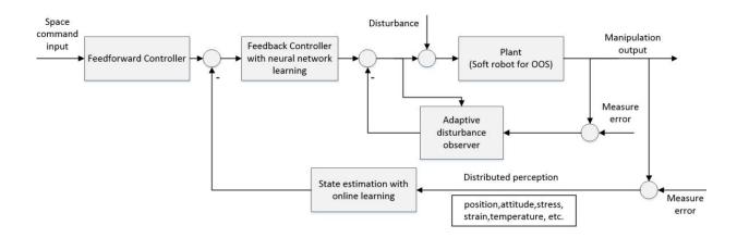
The block diagram of the manipulation system of the space soft robot for OOS. Credit: ©Science China Press
