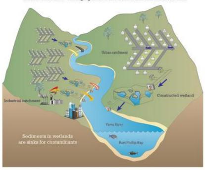
Melbourne Water has around 600 constructed wetland systems across Melbourne - managing stormwater from urban and industrial area.
