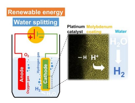
A high-resolution electron microscope image (right) of the platinum electrocatalytic layer coated with molybdenum. The platinum catalyzes the hydrogen-evolution reaction (left) in acidic medium from protons in the electrolyte while the molybdenum layer inhibits water-forming reactions. Credit: © 2017 KAUST
