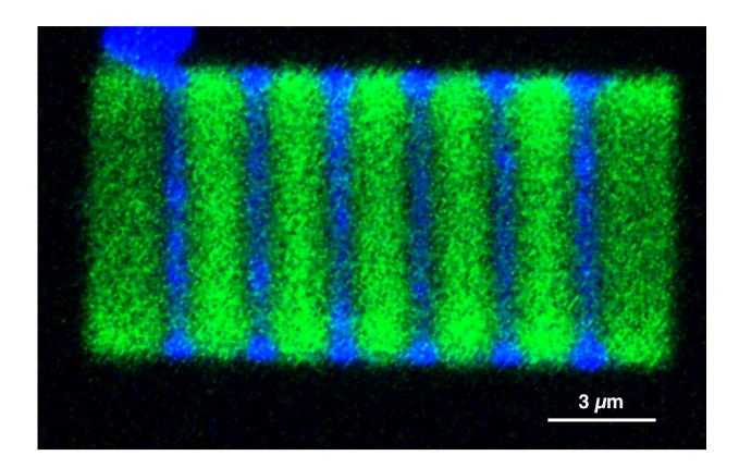
A 2-D plate showing alternating cesium lead chloride (blue) and cesium lead bromide (green) segments. Credit: Letian Dou/Berkeley Lab and Connor G. Bischak/UC Berkeley
