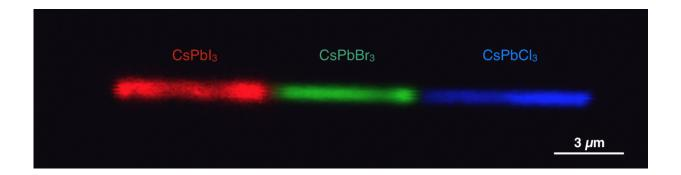
A cesium lead iodide-cesium lead bromide-cesium lead chloride heterojunction nanowire simultaneously emitting red, green, and blue light under UV excitation. Credit: Letian Dou/Berkeley Lab and Connor G. Bischak/UC Berkeley
