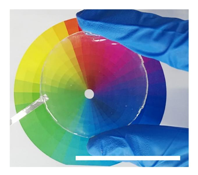
A circular soft and transparent triboelectric nanogenerator. Credit: Xiong Pu
