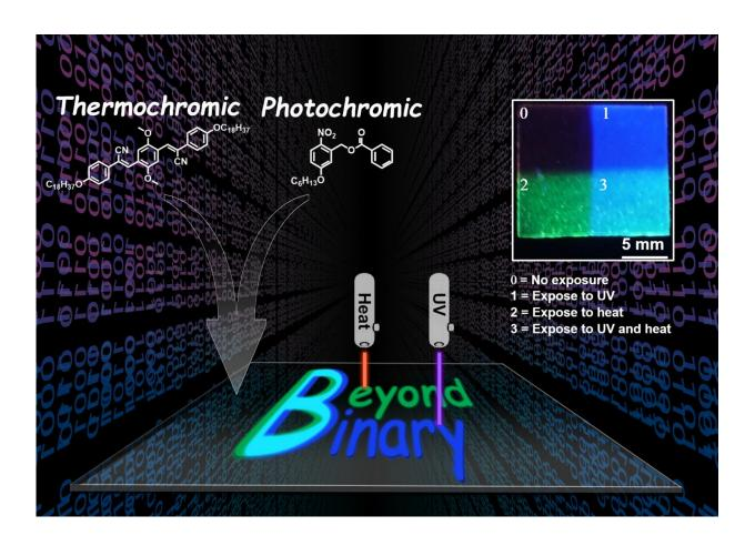
CWRU chemists developed a space-saving method to store digital data optically, using four-symbol, or quaternary code. The four symbols are the absence of color and three colors -- fluorescent green, ultramarine and cyan -- produced when dyes contained in a common polymer are exposed to heat, ultraviolet light or both. Credit: Emily Pentzer
