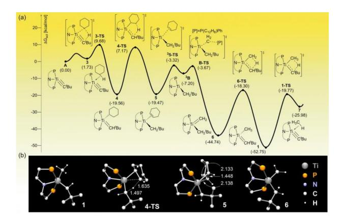
Computer generated energy profile of the reaction. Computer simulations can predict the intermediate components of the chemical reaction and how much energy is required to obtain them. Credit: Institute for Basic Science
