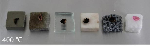
A porous, deformable sponge-like material made from ceramic nanofibers has remarkable heat resistance. Here, flower petals are heated atop 7-millimeterthick discs of varying materials. After heating the materials from the bottom at 400 degrees C, the petal atop the ceramic sponge is barely wilted, while the others are burnt to a crisp. Credit: Gao/Li/Wu/Brown University/Tsingua University
