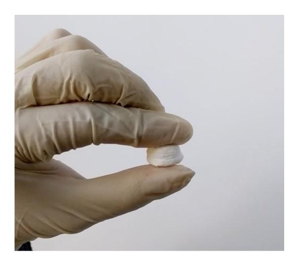
Researchers have developed a sponge-like material made from ceramic nanofibers. The material retains the heat resistance that makes ceramics useful in high-temperature settings, but is also highly deformable -- something that most ceramic materials are not. Credit: Gao/Li/Wu/Brown University/Tsingua University
