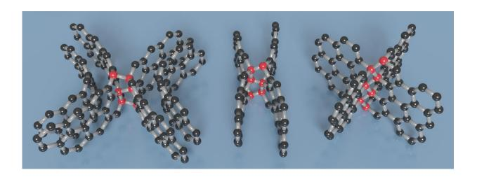
Visualization of the different types of diamond-like linkages (red spheres) formed at curved surfaces or between the layers of graphene (black spheres) in this new type of compressed glassy carbon. Credit: Timothy Strobel.
