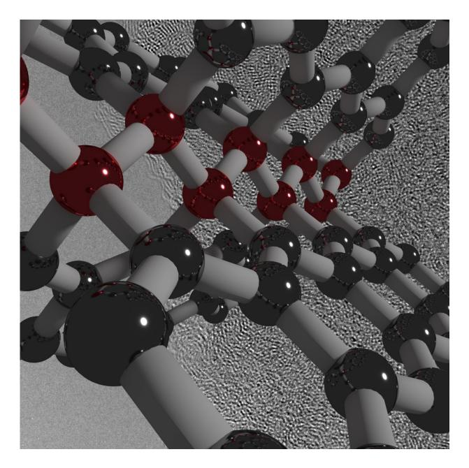
Visualization of ultrastrong, hard and elastic compressed glassy carbon. The illustrated structure is overlaid on an electron microscope image of the material. Credit: Timothy Strobel.
