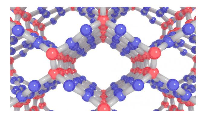
View through the channels of a mixed sp2 / sp3, interpenetrating graphene network in compressed glassy carbon. Graphene-like sheets (blue spheres) are crosslinked at diamond-like nodes (red spheres). Credit: Timothy Strobel
