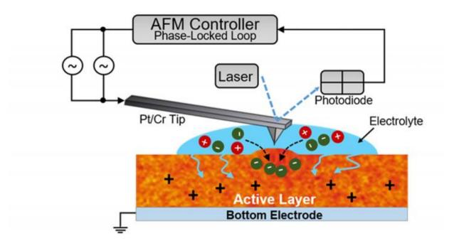
A schematic of the electrochemical strain microscopy technique used to measure which regions of the P3HT film could subtly swell to let in ion molecules. Credit: Rajiv Giridharagopal
