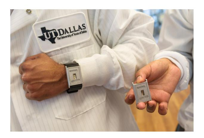
Researchers at the University of Texas at Dallas have developed a wearable diagnostic biosensor that can detect three interconnected, diabetes-related compounds -- cortisol, glucose and interleukin-6 -- in perspired sweat for up to a week without loss of signal integrity. The team envisions that their wearable devices will contain a small transceiver to send data to an application installed on a cellphone. Credit: University of Texas at Dallas
