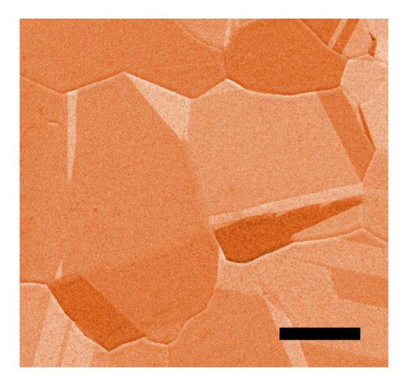
This false-color scanning electron microscopy image shows microscopic details on the surface of a copper foil that was used as a catalyst in a chemical reaction studied at Berkeley Lab's Advanced Light Source. The scale bar represents 50 microns, or millionths of a meter. Credit: Berkeley Lab
