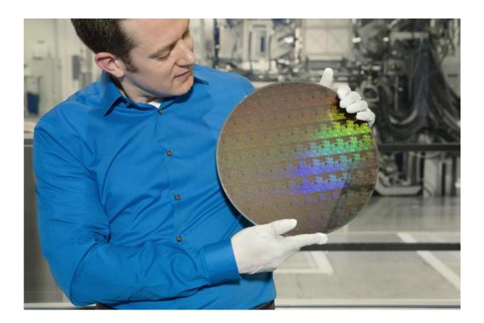
IBM Research scientist Nicolas Loubet holds a wafer of chips with 5nm silicon nanosheet transistors manufactured using an industry-first process that can deliver 40 percent performance enhancement at fixed power, or 75 percent power savings at matched performance. Credit: Connie Zhou
