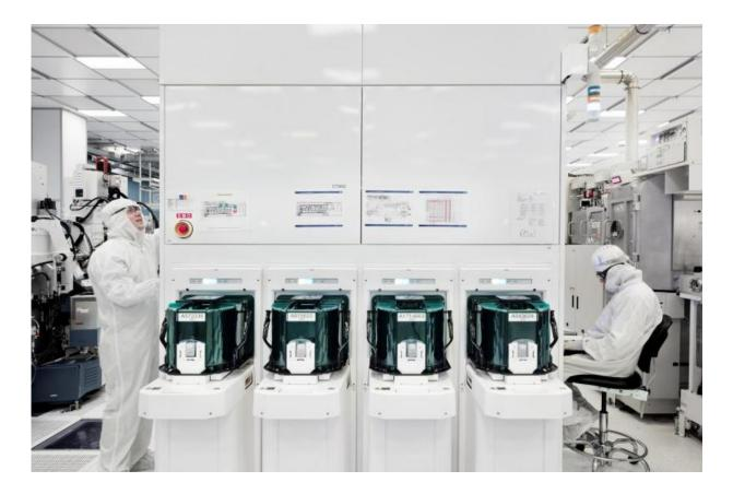
IBM scientists at the SUNY Polytechnic Institute Colleges of Nanoscale Science and Engineering's NanoTech Complex in Albany, NY prepare test wafers with 5nm silicon nanosheet transistors, loaded into the front opening unified pod, or FOUPs, to test an industry-first process of building 5nm transistors using silicon nanosheets. Credit: Connie Zhou
