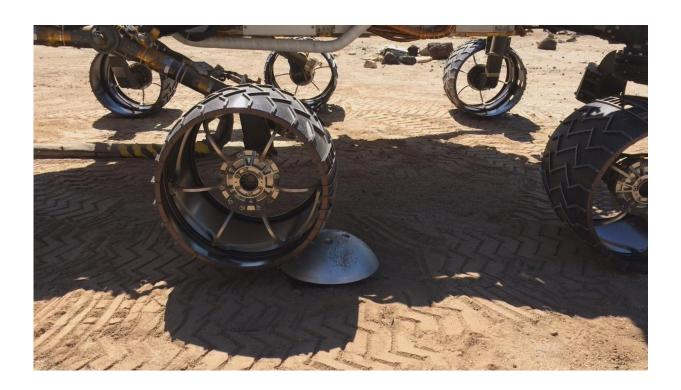
A "scarecrow" rover at NASA's JPL drives over a sensor while testing a new driving algorithm. Engineers created the algorithm to reduce wheel wear on the Mars Curiosity rover. Credit: NASA/JPL-Caltech
