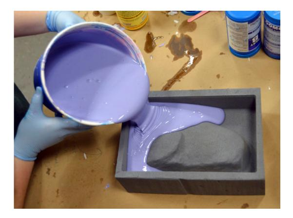
In this April 12, 2016 photo provided by Dartmouth College, silicone rubber is poured over a foam cast, created by using three-dimensional geometry, to create a mold for a hold that will be mounted on a climbing wall in Hanover, N.H. The hold, created by using three-dimensional geometry, is part of a replica of a rock wall created by tracking a climber's hand and foot positions and by estimating the contact forces. (Emily Whiting/Dartmouth College via AP)
