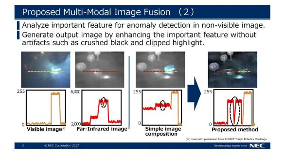
Credit: Obtained permission to use the severe environment simulator in the ImPACT Tough Robotics Challenge program.
