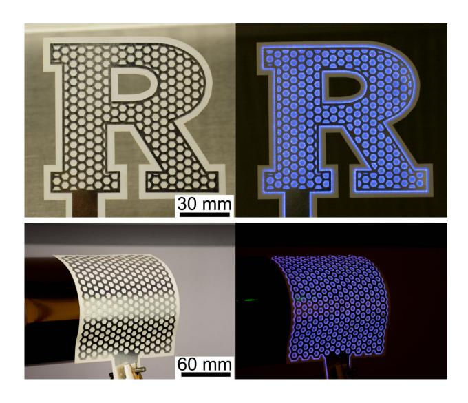
Paper-based plasma generators -- consisting of laminated assemblies of honeycomb-patterned, metallized paper -- are capable of sanitizing surfaces with 10 seconds of treatment. These devices are also customizable into varied planar geometries and bendable/mechanically flexible to conform to curved surfaces.
