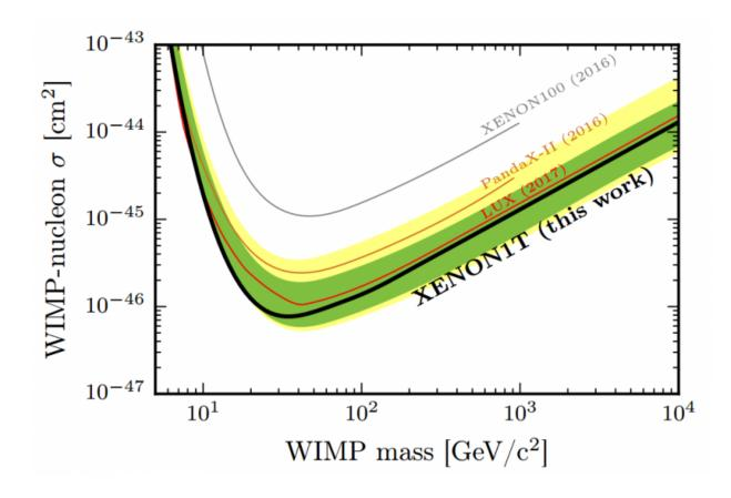
The spin-independent WIMP-nucleon cross section limits as a function of WIMP mass at 90% confidence level (black) for this run of XENON1T. In green and yellow are the 1- and  $2\sigma$  sensitivity bands. Results from LUX (red), PandaX-II (brown), and XENON100 (gray) are shown for reference. Credit: Purdue University
