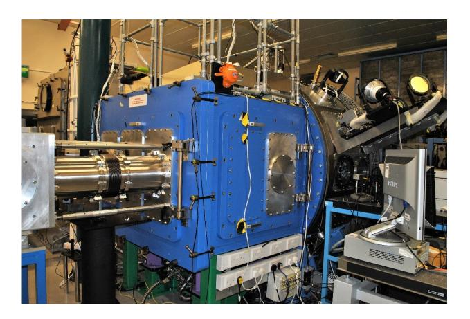
The Vulcan (TAW) laser target area at the Central Laser Facility, with the Raman amplification setup. Credit: University of Strathclyde
