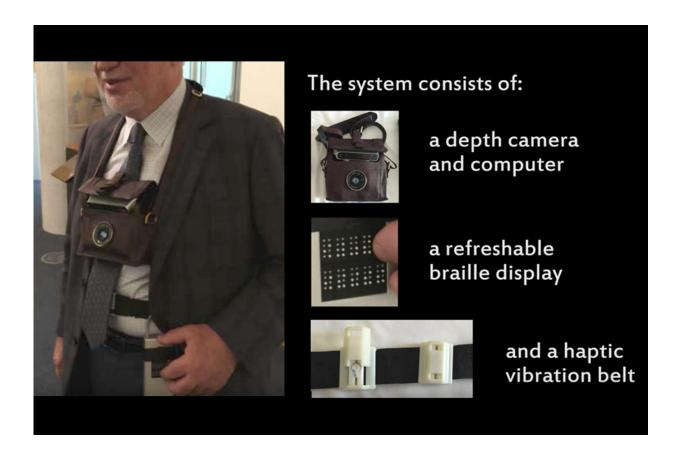
New algorithms power a prototype system for helping visually impaired users avoid obstacles and identify objects. Credit: Massachusetts Institute of Technology
