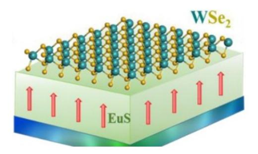
A two-layered heterostructure, with a 10 nanometer thick film of magnetic EuS (europium sulfide) on the bottom and a single layer (less than 1 nanometer) of the transition metal dichalcogenide WSe2 (tungsten diselenide) on top. The magnetic field of the bottom layer forced the energy separation of the valleys in the WSe2. Credit: *Nature Nanotechnology*.
