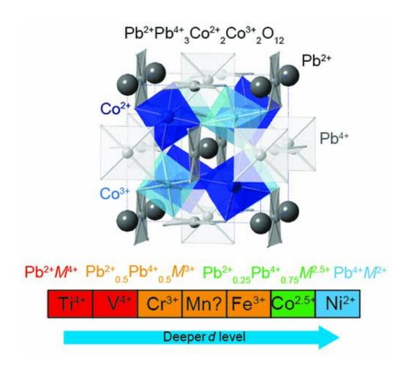
Crystal structure of Pb2+Pb4+3Co2+2Co3+2O12 where Pb and Co have charge orderings despite the simple PbCoO3 chemical composition and the valence distribution changes for PbMO3 (M: 3d transition metal). Credit: *Journal of the American Chemical Society*
